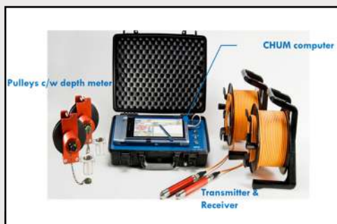
The ultrasonic cross-hole (CSL) Test Apparatus
