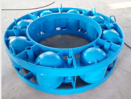
A typical bidirectional cell for bored pile
