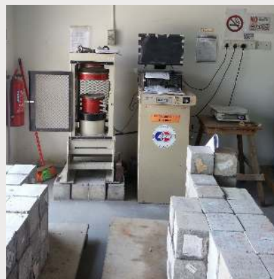
Concrete Cube Test
