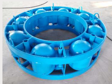
A typical bidirectional cell for bored pile
