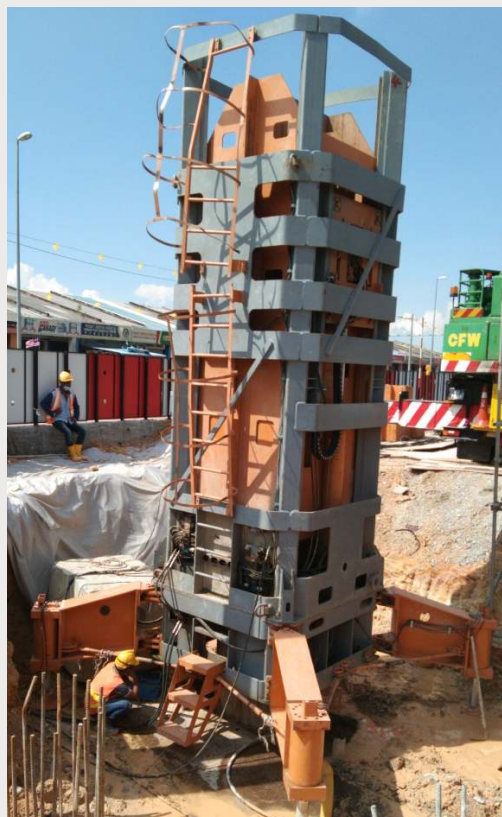
HSDLT with 60tonnes of hammer
