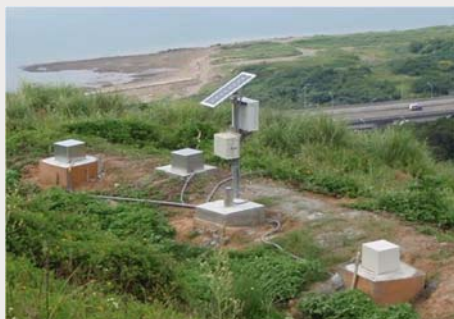
Instrumentation and monitoring for slope stability
