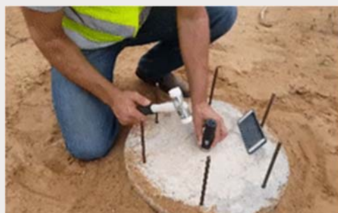
Low strain dynamic pile test
