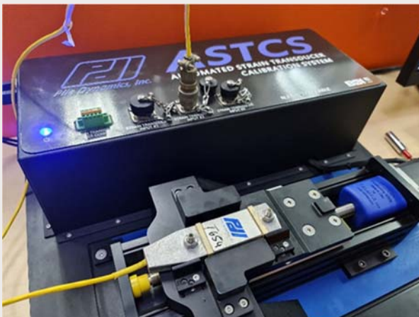
The overall view of ASTCS calibrator.
