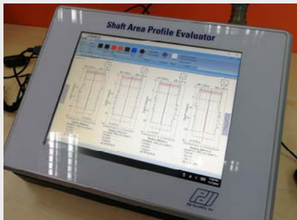
The mobile read-up unit of SHAPE equipment
