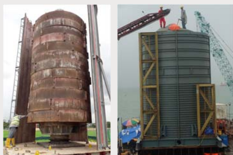
Setup of Statnamic Test
