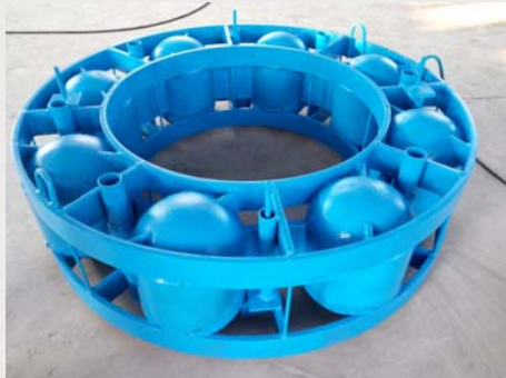
A typical bidirectional cell for bored pile
